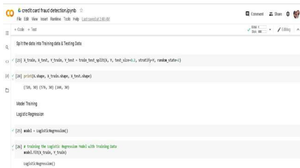
Figure4: The logistic regression model is trained using the training data After training the data with logistic regression finding the accuracy of both the datasets.
